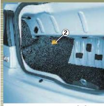
Luggage compartment light 2 Press tab 3 to release the bulb holder and gain access to the bulb 4.
