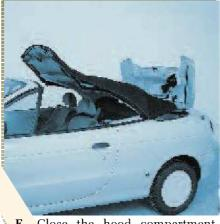
E - Close the hood compartment cover. Make sure it is properly locked.
