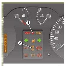
Warning light to indicate that the system is not operating correctly
