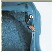
Unclip bulb holder **3** by pressing the two tabs.
