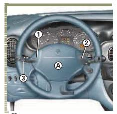
Press buttons 1 or 2 on the steering wheel boss A.
